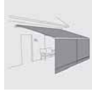
Drop curtain awning
